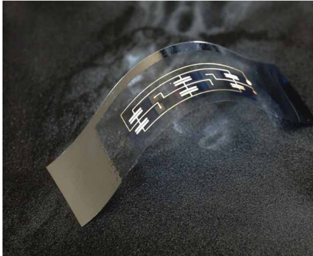
First all-printed plastic circuit Lucent Technologies
