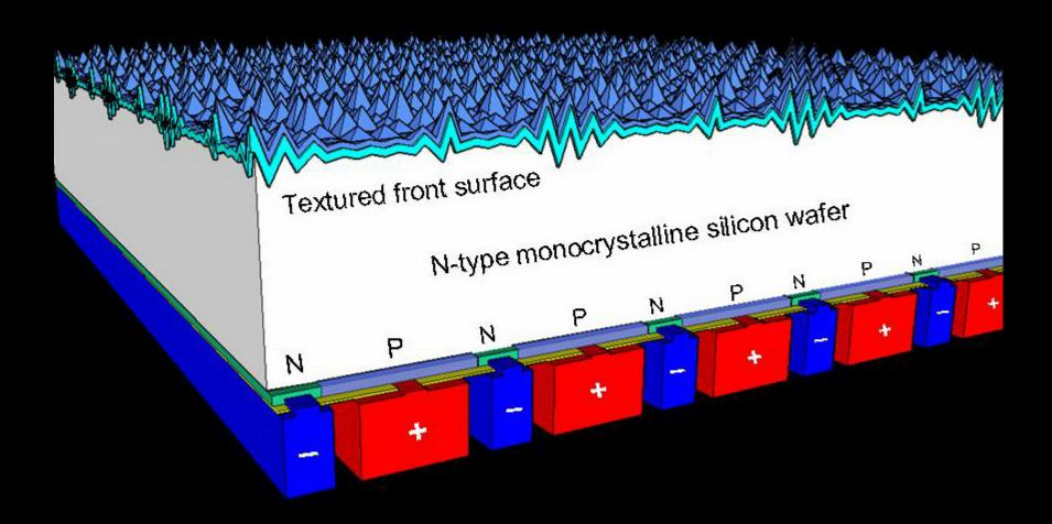
By locating all of the electrical contacts on the back surface, SunPower is able to achieve conversion efficiencies up to 50% higher than conventional solar cells.
